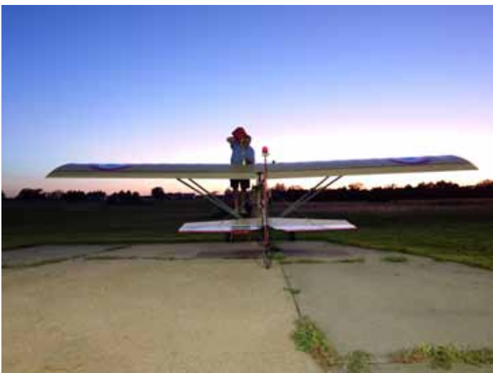
Wing tanks hold 10 gallons and fuselage tank holds 1-1/2 gallons of 91 octane auto gas. Photo taken by Tom Balzer, hangar owner where I rent space along with several other pilots.
