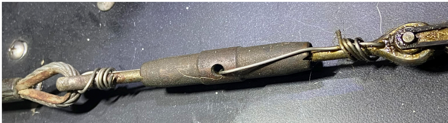
FIGURE 7-27. Assembling and securing clip-locking turnbuckles
