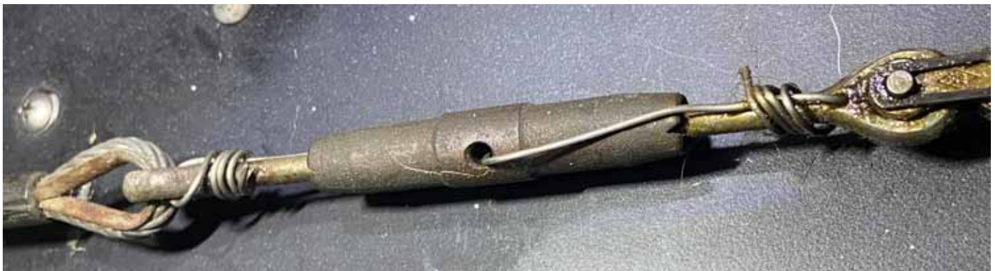
FIGURE 7-27. Assembling and securing clip-locking turnbuckles
