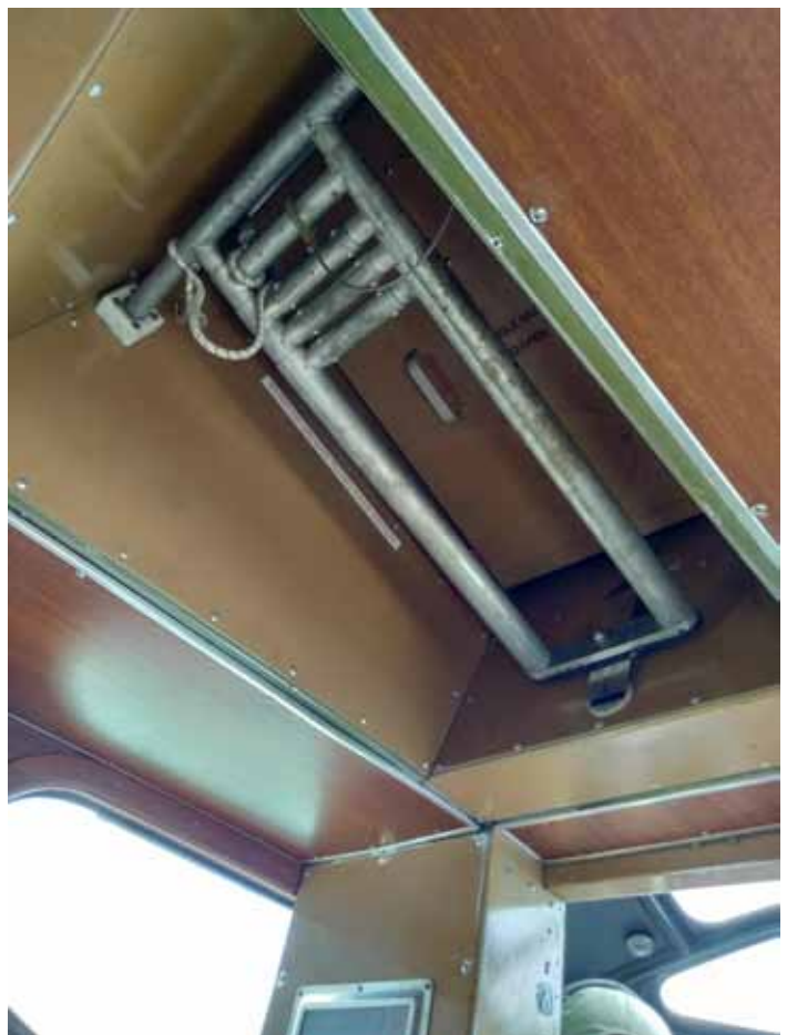
Ladder and ceiling hatch providing access to the wing for refueling
