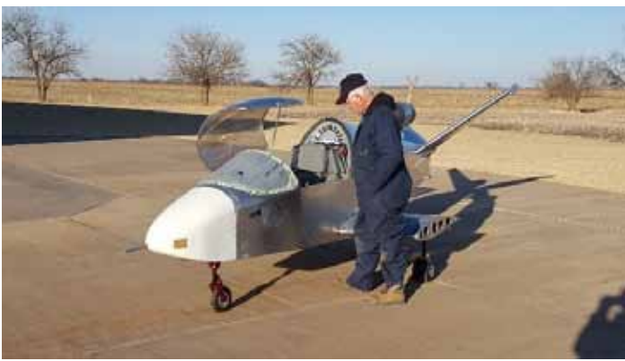
First taxi test was on the driveway at home before installation of the wings.
