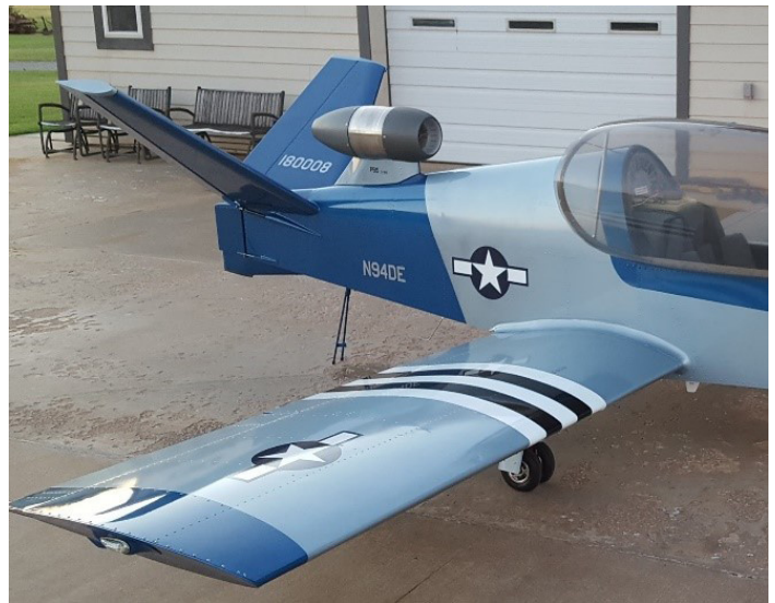
Pneumatic tail stand for parking without the pilot since the plane is tail heavy with the rear engine if the pilot is not seated.
