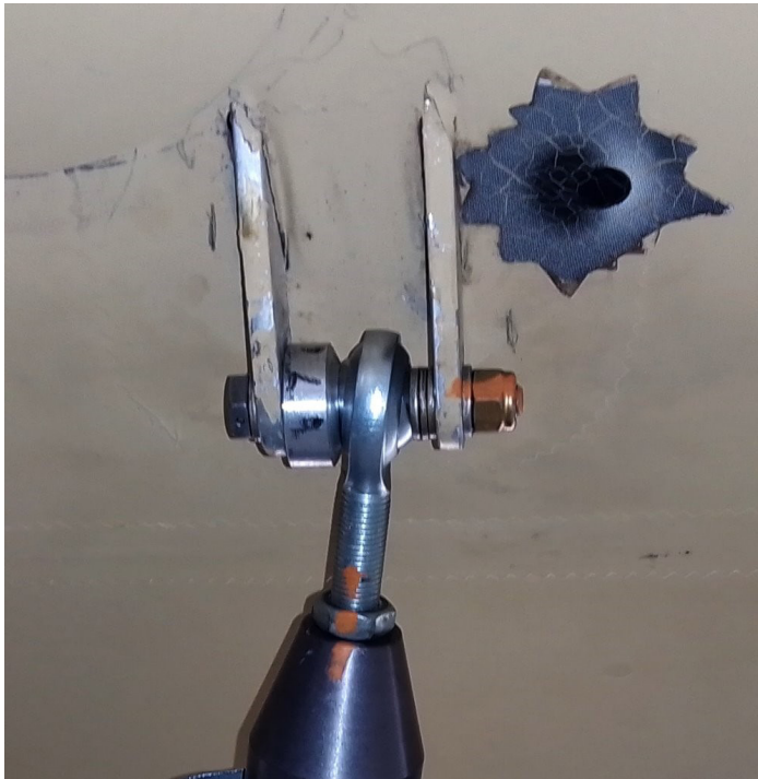
Aft strut attach point completed. The rod end bearing compensates for the compound angle.
