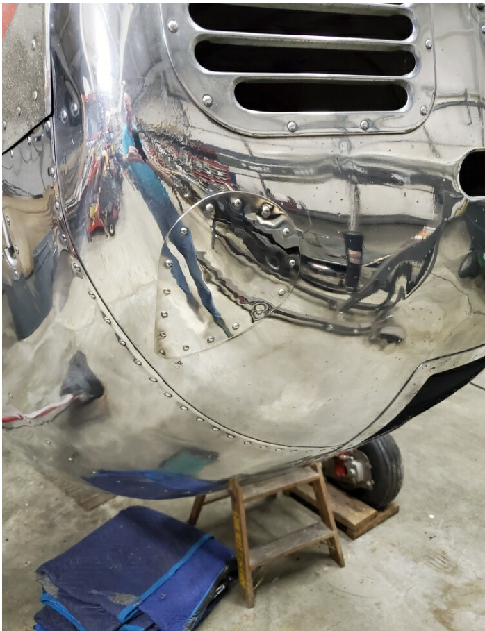
Patches on expensive cowl areas covering small "wear holes" due to engine mounts fatigue lowering engine and touching cowl.
