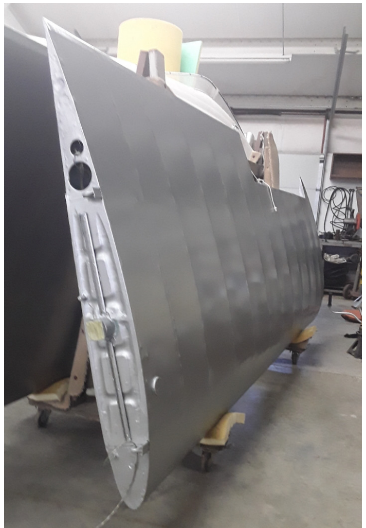
Below: Finished wings with several coats added for UV resistance.
