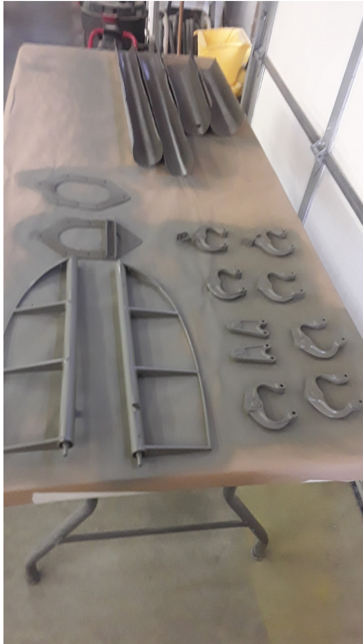
PT26 elevator parts cleaned/painted. Ready to start rebuilding it!
