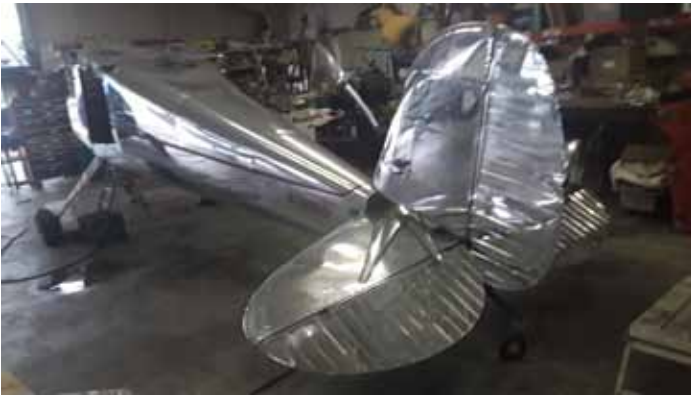
Most of the polishing has been done, using a product called "Nuvite Aluminum Polish"
