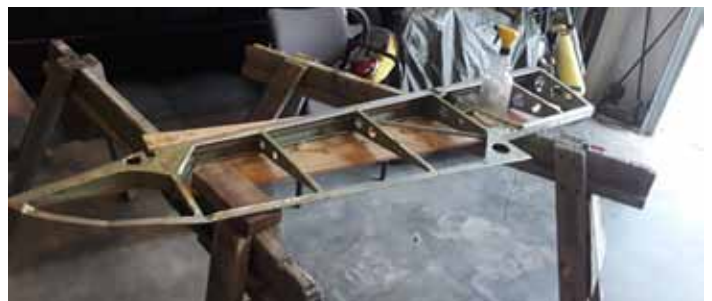
Left aleron (PT26) w/ fabric off but, before cleaning.
