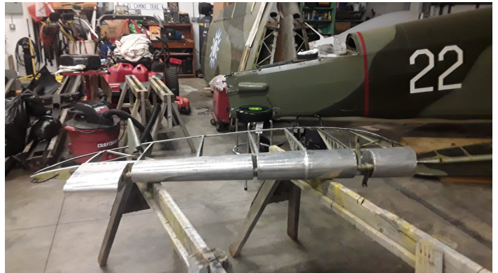
Two Trim tab frames (just bead-bead-blasted clean)
